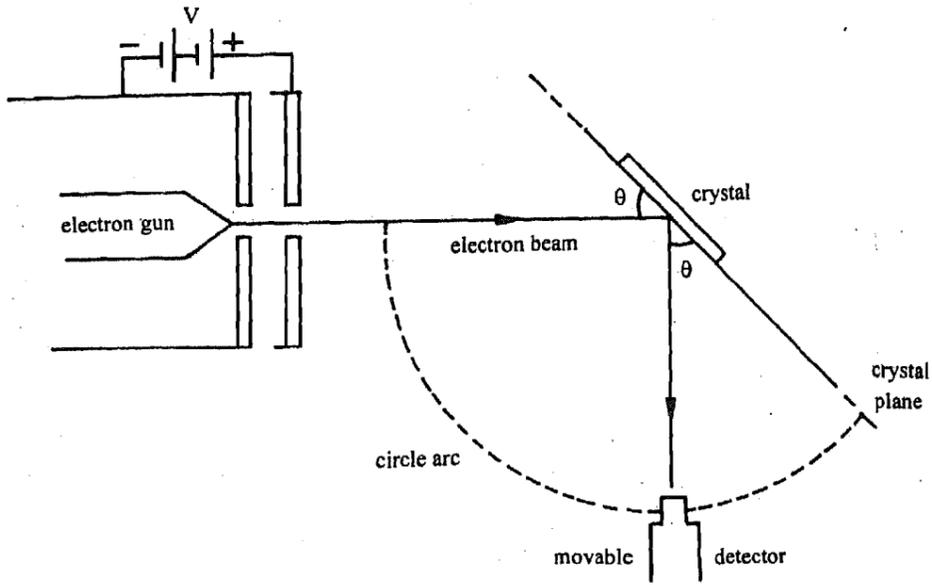
Fig. 4.9 : Schematic diagram of Davisson-Germer Experiment.
