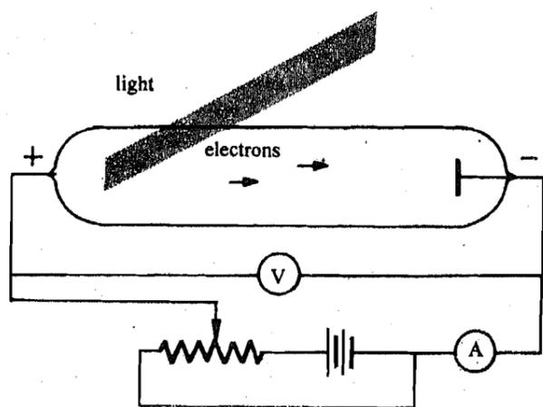
Fig. 4.3 : Schematic diagram of the apparatus for photoelectric effect.
