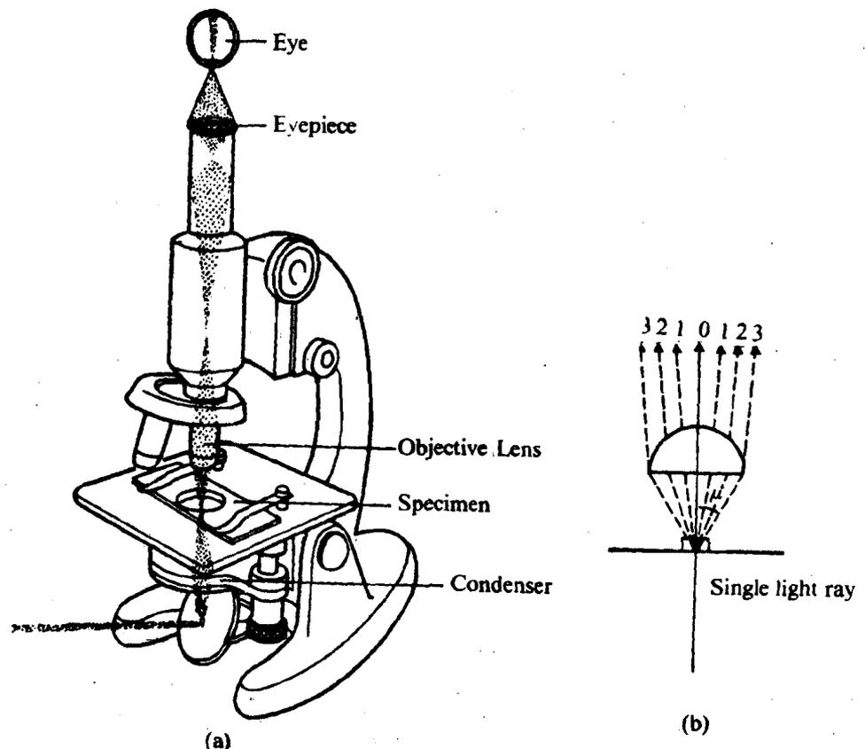
Fig. 2.1 : a) Light path in a compound microscope. The objective lens is near the specimen and the observer looks into the eye piece at the upper end of the tube of the microscope. The specimen is beyond the focal point of the objective lens.
