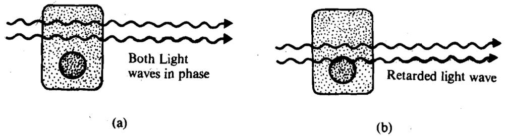
Fig. 2.3 : a) When two light waves are passing side by side, through a cell and if they have encountered the same refractive index and thickness of medium, they will emerge in phase.
