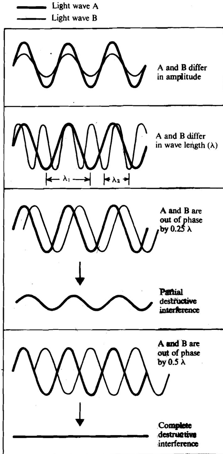
Fig. 2.4 : Properties of light waves that result in partial and complete destructive interference.
