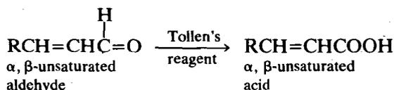
In this reaction, a shining coat of silver metal gets deposited on the glass surface of the reaction vessel. So it can be used as a test to detect the presence of aldehydes. Mirrors are also prepared commercially in this way.
