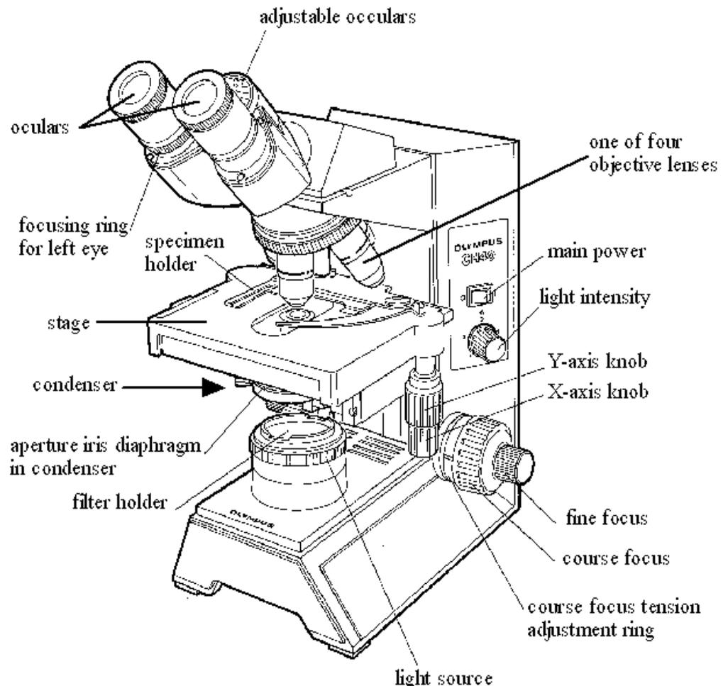
Figure 5.1: Labelled diagram of a compound microscope
