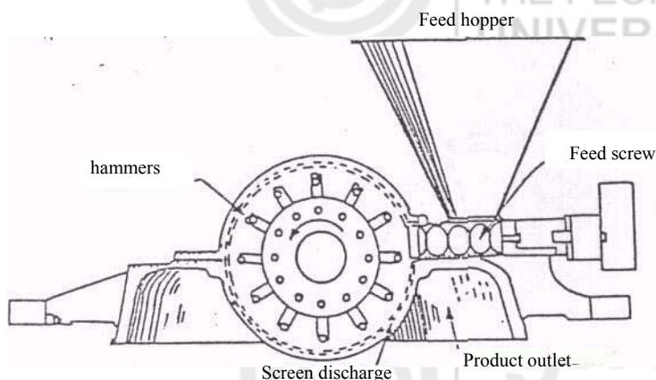
Figure 9.5: Sectional view of hammer mill
