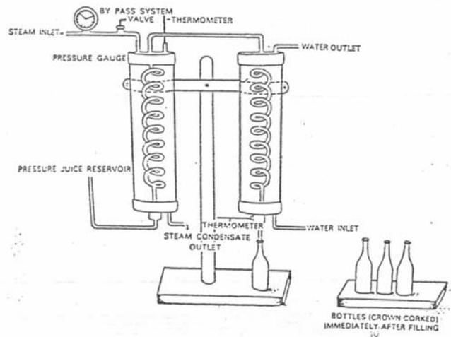
Figure 9.10: Schematic representation of a flash pasteurizer
