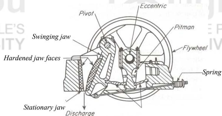
Figure 5.1: Jaw crusher
