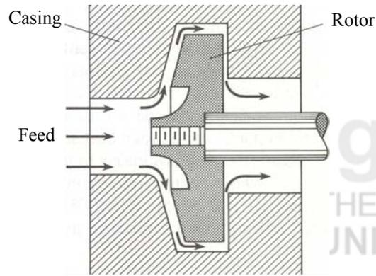
Figure 5.9: Schematic drawing of colloid mill
