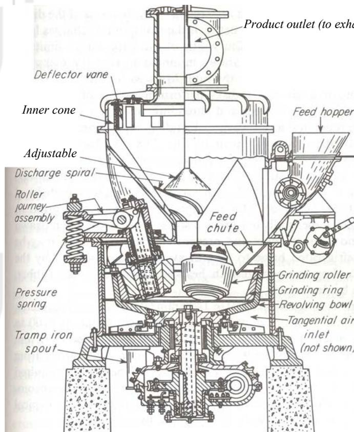
**Figure 5.6: Roller mill**
