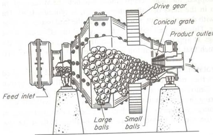
**Figure 5.8: Conical ball mill**
