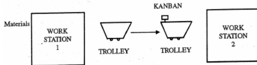
Work station (WS-2) is the customer, he will decide when he needs the next lot of material. For this, he will transfer the Kanban to WS-1 only when its incoming trolley is nearly empty - the worker at WS-1 cannot transfer the material until he receives the Kanban from his customer stage. By controlling the no. of Kanbans in the production process, work-in-progress is reduced and materials arrive into the next workstation just-in-time.
