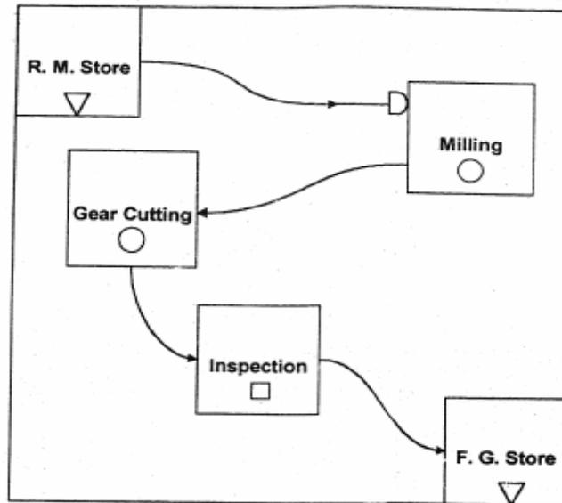
Figure 9.5 : Flow Diagram (Gear Making)
