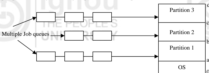
Figure 6: Multiple Partition System
