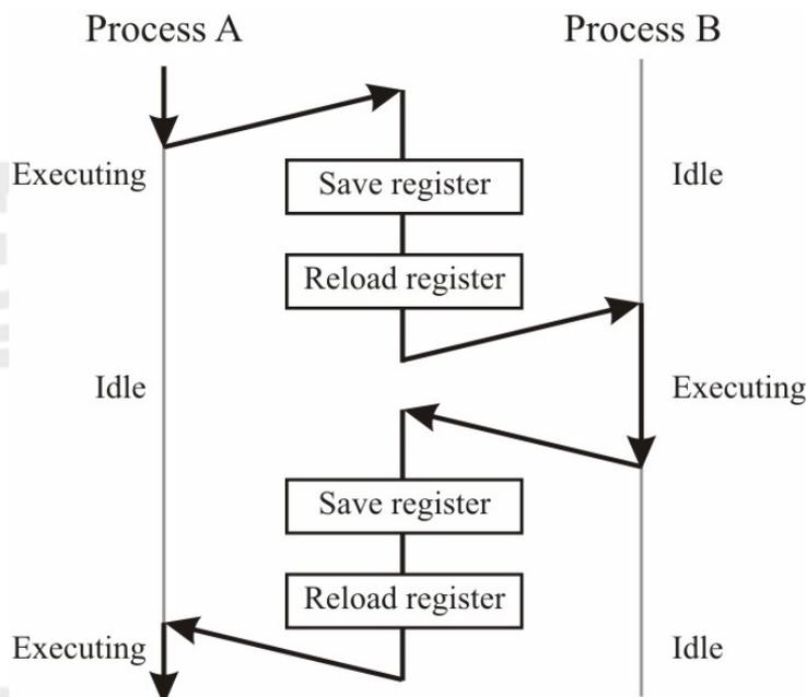
Figure 3: Process Switching between two processes
